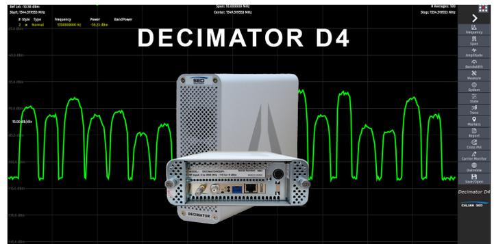
The Portable Decimator D4 uses state of the art digital technology and Fast Fourier Transformations to make fast and accurate measurements. With a very low noise floor and large dynamic range, it is well-suited to measure any type of satellite, cable or terrestrial wireless carrier, including very small carriers, beacon signals and for carrier monitoring applications.
